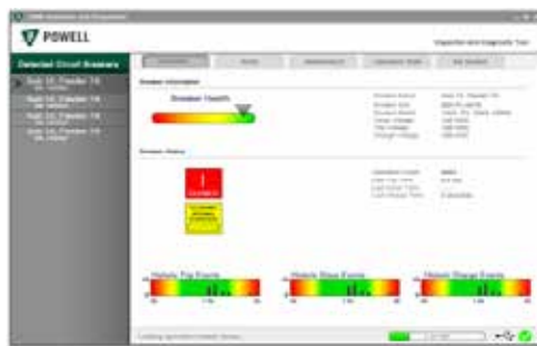
Example of Diagnostics Software Pages Circuit Breaker Overview - Health Indication Graph of a raw profile - trip/close/charge Processed data - calculated results and limits
