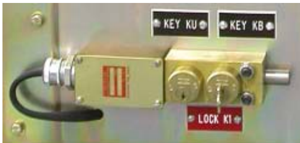
Figure 62. Key KB is Captive and Key KU is available
