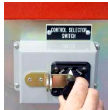
Figure 63. Verify the Control Selector Switch is in the OFF Position
