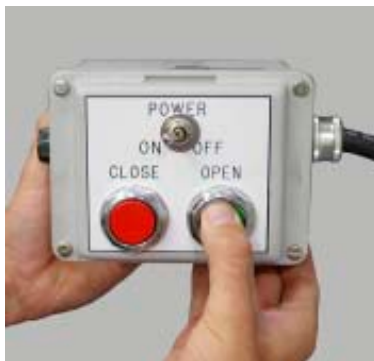
Figure 80. Depress the Remote Operating Station OPEN Push Button
