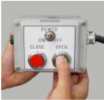
Figure 96. Depress the OPEN Push Button Switch on the Remote Operating Station
