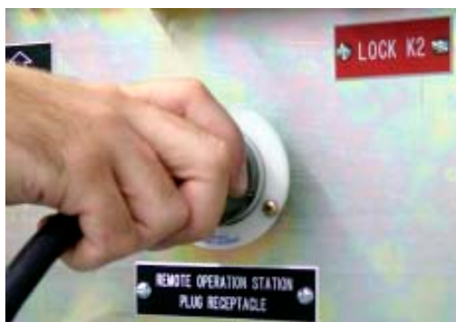
Figure 45. Disconnect the Remote Operating Station Umbilical Cord
