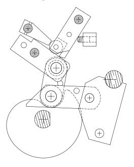
a) Breaker Open - Spring Charged - Links Reset
